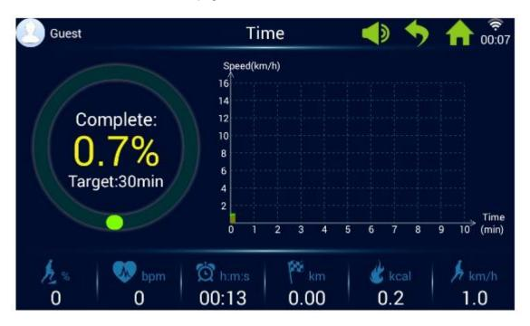
During the process of time countdown, click anywhere of the screen to enter incline and speed adjustment page as below. Press -Incline+ and -Speed+ button to adjust the speed and incline.
