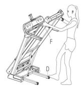
• To transport, hold the treadmill from F position and tilt until the wheels are able to move on the ground.
