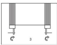
**WARNING:** To prolong product lifespan, we suggest switch off the treadmill for about 10 minutes after 2 hours of exercising. Too loose or too tight belt could damage this machine. Keep a suitable tightness. Grasp the running belt and pull it up to certain distance until you cannot pull it anymore. If the distance is between 50-75 mm, the tightness is proper.
