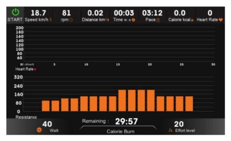
Work-Out: First choose a certain program and then finish setting movement data. There are 16 sections inside for each program. And each section time = setting time/16. The resistance for each section is as described below.
