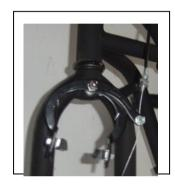
Note: If additional brake adjusting is required, you can bring the brake rubbers closer to the wheel rim by turning the adjusting screw counter-clockwise . To make the brake rubbers further from the rim. turn the adjusting screw clockwise.
