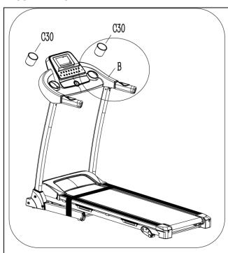
Put the bottle holder (C30) into the console (B) kettle slot.
