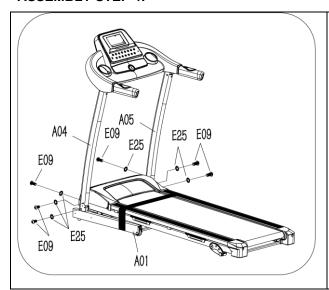
Use the 5# Allen wrench (B08) and M8\*15 bolt (E09) and lock washer (E25), lock the left & right upright tube (A04, A05) onto main frame (A01).
