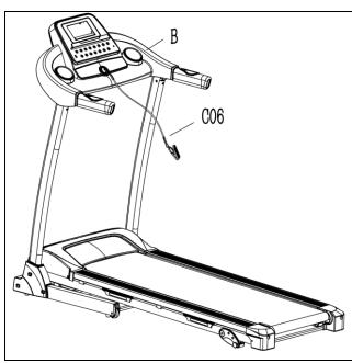
Before running, please insert the Safety Key (C06) into the magnetic area of the Console (B) and fasten the safety key clip (C06) with your clothes.
