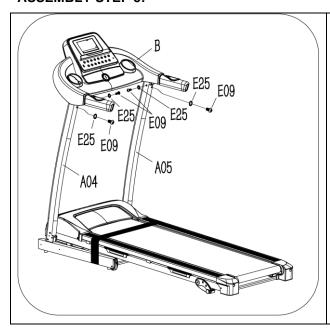
Use the 5# Allen wrench (B08) and M8\*15 bolt (E09) and lock washer (E25), lock the console (B) onto the left and right upright tube (A04, A05).
