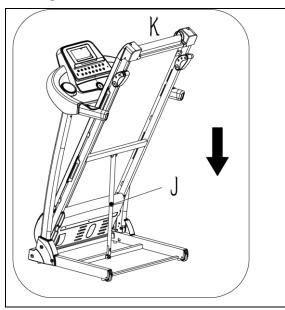
Support place K with a hand, press the frame slightly, then kick the place J, and the base frame will fall down automatically.
