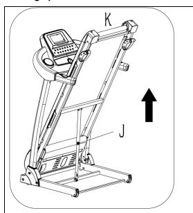
Support place K with a hand, and then pull up in the direction of the arrow, until hearing that the CYLINDER (J) is locked into the round tube.
