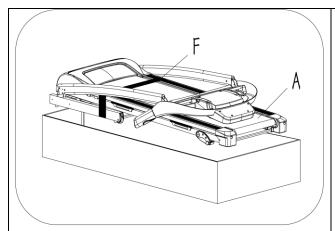
Open the carton and remove contents. Place the Main Frame (A) on level ground, ensure that you have a work area that is clean and has adequate space. Please do not cut packing belt (F) before you finish assembly.
