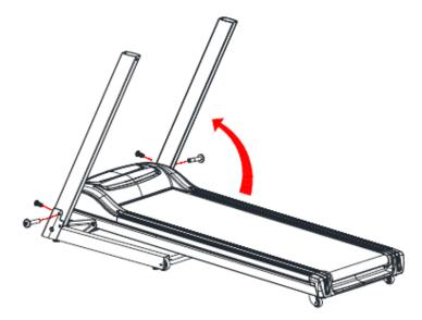
**Step3:** Put the handle bars in a horizontal line (in the direction shown), then connect console B and the upright post with 4 pcs of Allen C.K.S: half head screws M8x15 (lock the bolts).
