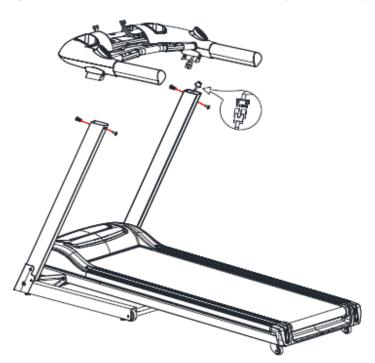
**Step 4:** Put console A on the treadmill and connect the wires well. Use the Allan socket full thread screws M6x25 to tighten the console.
