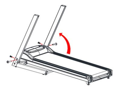
**Step3:** Put the handle bars in a horizontal line (in the direction shown), then connect console B and the upright post with 4 pcs of Allen C.K.S: half head screws M8x15 (lock the bolts).
