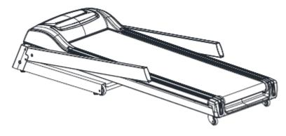
**Step 2:** Insert the upright post into the clamping ring on both sides of the main frame with Allen C.K.S. half head screw M8x50x20 and Allen C.K.S. full thread screw M8x15 (without lock for now).
