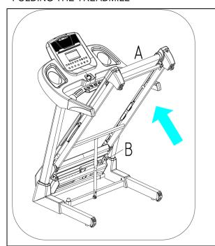
Place your hand at the end of the running deck (position A) and lift up the main frame (A02) until the air pressure cylinder (B03) locks (position B).
