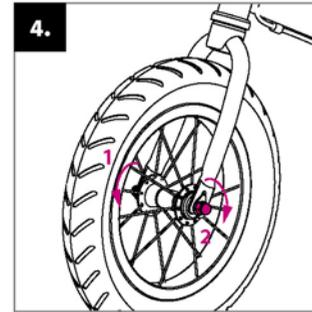
Place the wheel into the front fork so that it is well-centered and tighten the nuts (1, 2). (For easier installation you can turn the running bike upside down).
