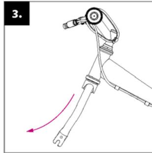
**Front wheel installation:** make sure the front fork of the running bike is well positioned (the bending of the fork faces forward).
