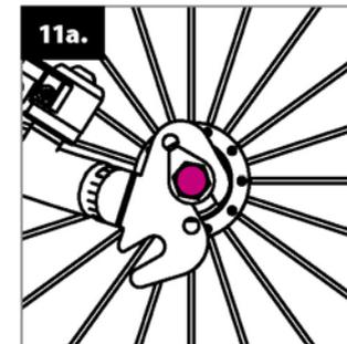
Yedoo **TOO TOO ALU** is equipped with double dropout at the rear fork, which enables a bigger range of seat height. The upper dropout is meant for lower seat position.
