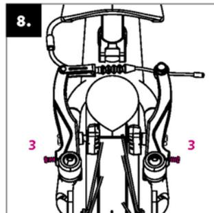
In case the brake pad is touching the wheel when turning, symmetrically adjust the distance of brake arms by the tightening screws (3).
