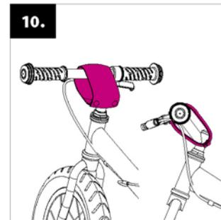
**Protective pad installation:** place the soft protective pad from washable nylon over the handlebar stem.
