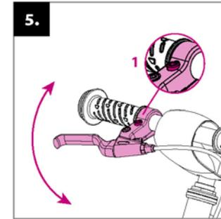
**Adjustment of brake levers:** incline the brake levers correctly by loosening the screw on the sleeve (1).
