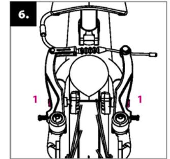
**Adjustment of brake:** before adjusting the brakes, inflate the tires according to the values on their side (ideally between 1,3 and 1,8 bars). Check that the brake pads fit tightly on the rim sides. Their position can be adjusted via the screws (1). The pads shall not touch the tires.
