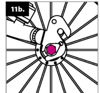
The lower dropout, on the contrary, enables the seat to be positioned higher than usual. Warning: after each position change, readjust the brakes.
