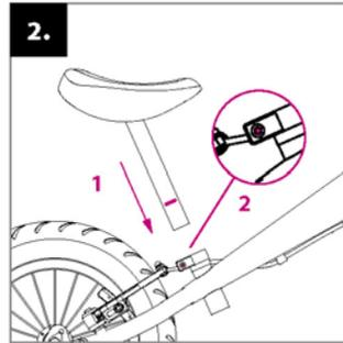
**Seat installation:** put the seat tube into the frame (1) of the running bike, adjust the desired height (do not exceed the maximum mark) and tighten the sleeve screw (2).
