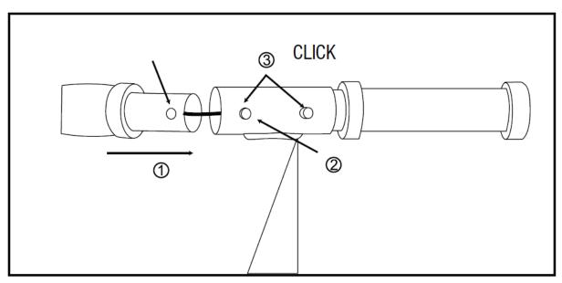
WARNING: Failure to properly lock the push pins can result in handlebar movement and a loss of control when using the product.
