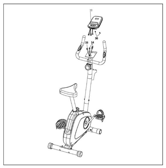
Attach the Console (10) to the Handlebar Upright (2) using 2 x M5 x 10mm Screws (30). Connect the Upper Link Wire (33) and Pulse Sensor Wire (14) into the back of Console (10).
