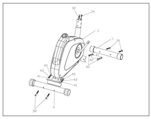
Attach the Front and Rear Stabilizer (5 & 6) to the Main Frame (3) with 4 x M8 x 75mm Carriage Bolts (38), 4 x M8 Curved Washers (41), 4 x M8 Spring Washers (42) and 4 x M8 Dome Nuts (40).
