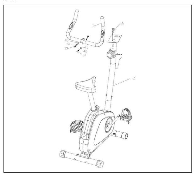
Fit the Handlebar (1) onto the Handlebar Upright (2) with 2 x M8 x 25mm Allen Bolts (13), 2 x M8 Curved Washers (41), 2 x M8 Spring Washers (42).
