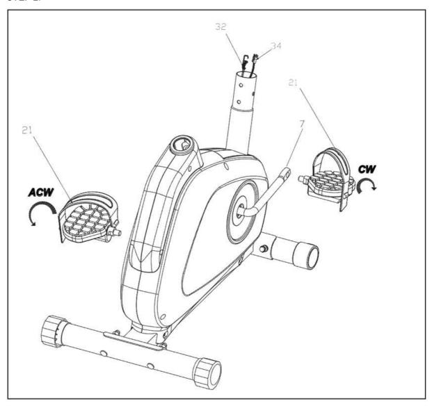
Assemble the Pedals (Left and Right) (21L & 21R) to the Pedal Crank (7) (see note). Both Pedals MUST be tightened securely otherwise damage may occur to the Crank. Fit the Pedal Straps (Marked L and R) ensuring a snug, but not tight fit with your normal footwear.
