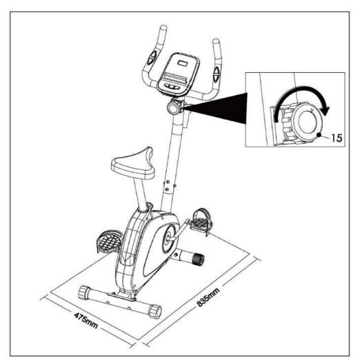
To adjust the pedaling resistance during use, start by turning the Tension Controller Knob (15) fully COUNTER-CLOCKWISE at the start of your workout. Gradually increase the pedaling resistance by turning the Tension Controller Knob CLOCKWISE as required.
