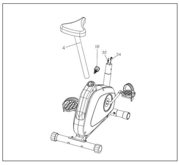
Slide the assembled Saddle Stem (4) into the Main Frame (3), select the desired height to allow for a knee bend at the bottom of the pedaling action and secure in place with the Saddle Adjustment Knob (18).
