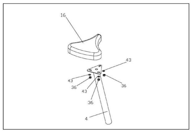
Remove the 3  $\times$  M8 Nylon Locknuts (36) and 3  $\times$  M8 Flat Washers (43) from the underside of the Saddle (16).
